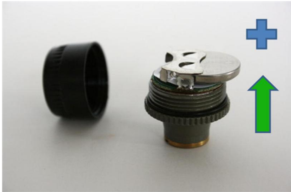
TMG400C transmitter and battery placement
