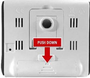
3. Move the battery (LR44) from the right slot to the left slot.
