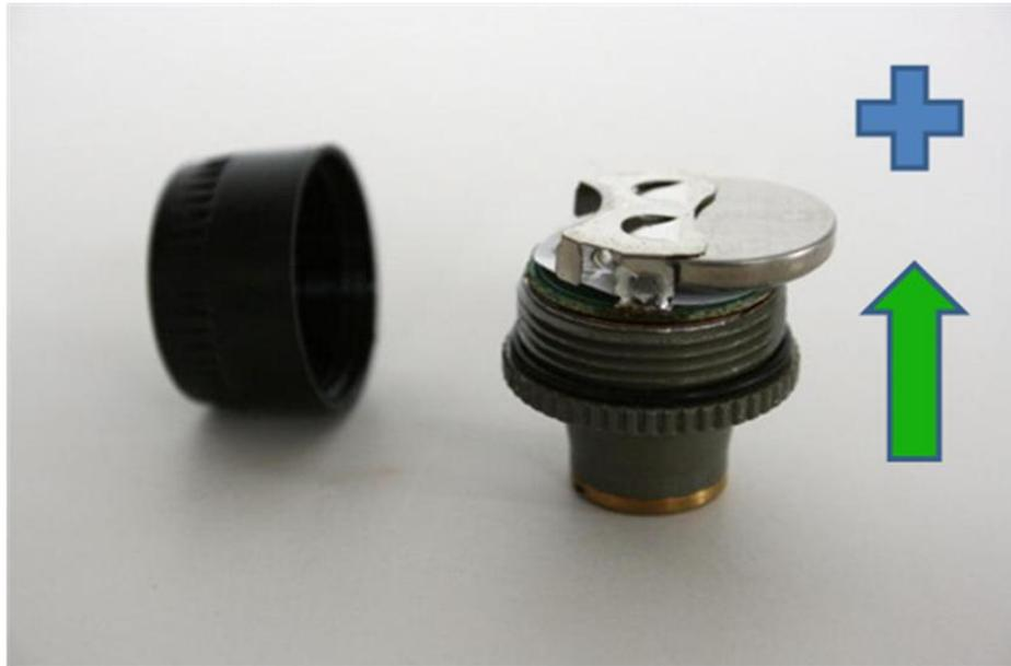
**TMG400C transmitter and battery placement**
